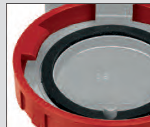
All gaskets are moulded directly on the cover and at the coupling point with the grip. Grip closing is by means of metric screws and metal inserts, making tightening easier and allowing for unlimited inspections and closings.
