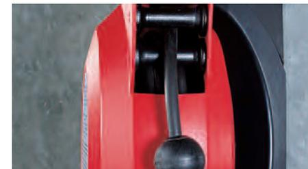
**Wall mounting bracket:** allows the Autoroller to be secured onto any vertical surface. There is housing for the safety transformer and two cable clamps are fitted onto the rear of the bracket. When correctly installed, the bracket allows the unit to swivel 310° in the direction of the cable pull.
