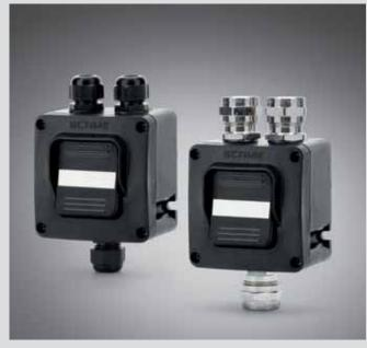
Control devices in the ROCKER-EX[GD] Series used to control lighting systems in environments with classification Ex zone 1/Gb -2/Gc (due to the presence of gases, vapours and mists in group IIC) and/or zone 21/Db - 22/Dc (due to the presence of the combustible dust in group IIIC). They are available as an ON-OFF switch, two way switch and 2 poles push-button. Made from a sturdy material charged with glass-fibre, they guarantee functionality in the most adverse weather conditions.
