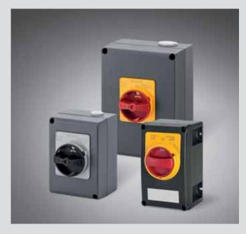
ISOLATORS-EX is a range of load-break switches/disconnectors with a switching and isolating functions, built in accordance with the standard EN 60947-3. Able to satisfy all installation needs, they are available in two versions in terms of the material used for the enclosure: thermoplastic or aluminium. They have a category of use up to AC-3 and are available in different versions for general use (handle in black) or for emergency control (high-visibility handle in red/yellow)
