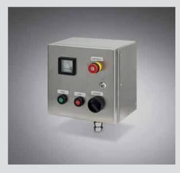
The ZENITH-S Series can be customised as a control station. The control stations can be assembled to house a broad range of actuators and components with separate ATEX-IECEx certification, including buttons, indicators, selectors, analogue instruments, etc... It is also possible to customise units including MCB, MCBO, RCD, transformers, disconnectors, fuses, timer or thermal relays, all with "Ex db eb" certification.
