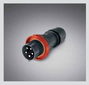
Plugs in the OPTIMA-EX Series are suitable for use in environments with classification Ex zone 22/Dc (due to the presence of the combustible dust in group IIIC) in the self-certification scheme.
