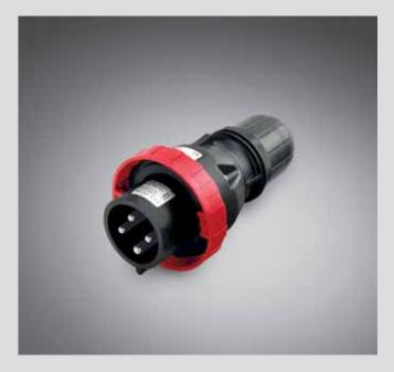
Plugs in the OPTIMA-EX[GD] Series (Ex eb) are suitable for use in environments with classification Ex zone 1/Gb -2/Gc (due to the presence of gases, vapours and mists in group IIC) and/or zone 21/Db - 22/Dc (due to the presence of the combustible dust in group IIIC). They are compatible with the interlocked sockets in the ADVANCE-GRP[GD] Series, but can be connected, when in a "safe zone", to any socket compliant with the industrial standard IEC/EN 60309 having the same polarity.
