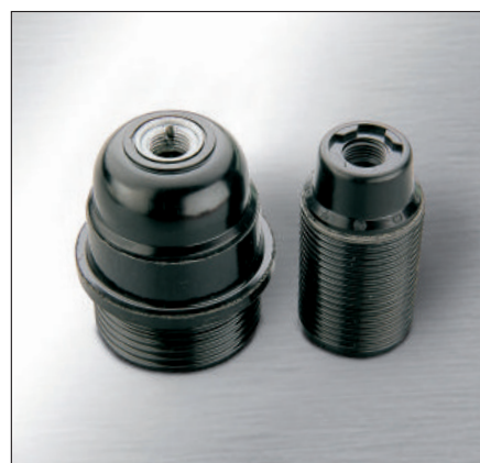
Thermoset lampholders: left, with E27 coupling, partly threaded skirt and metal nipple; right, with E14 coupling, fully threaded skirt and moulded thread.
