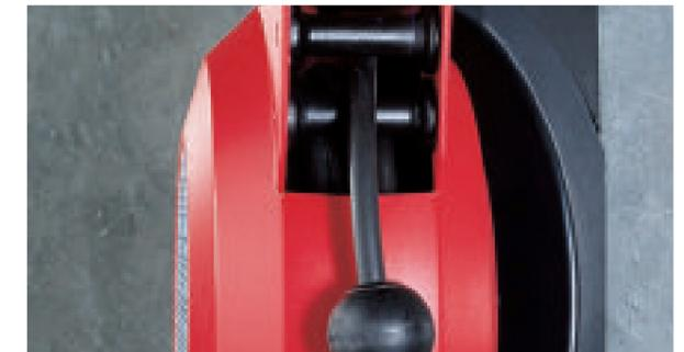
**Wall mounting bracket:** allows the Autoroller to be secured onto any vertical surface. There is housing for the safety transformer and two cable clamps are fitted onto the rear of the bracket. When correctly installed, the bracket allows the unit to swivel 310 ° in the direction of the cable pull.
