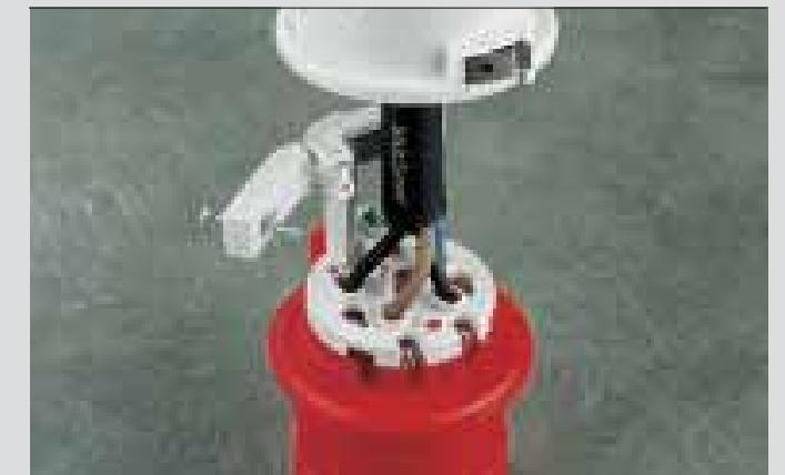
The cable clamp is located inside the housing to protect it from damage. The cable is clamped by tightening one single screw using a screwdriver for either single-slotted or cross-slotted screws. To assist wiring operations, the cable clamp is equipped with a “catch” to keep it open and to leave room for the hands when installing.
