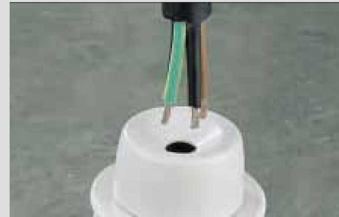
The cable is inserted into the cable sleeve on IP44 versions and into the cable gland on IP67 versions. There is no need to adjust the cable sleeve to the cable size.
