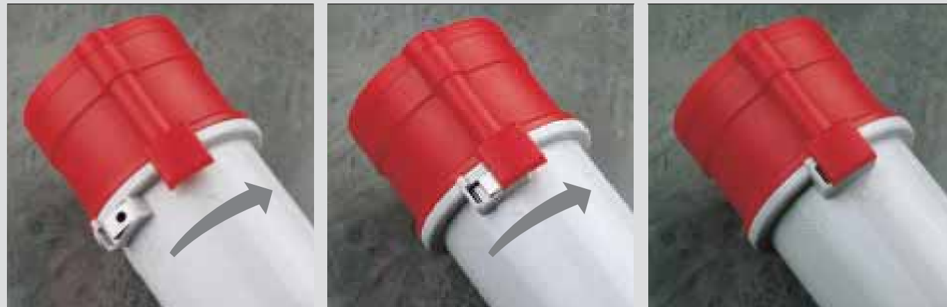
The spring on the side of the grip holds it fast against the insert. By twisting the assembly, the spring snaps into its housing.
