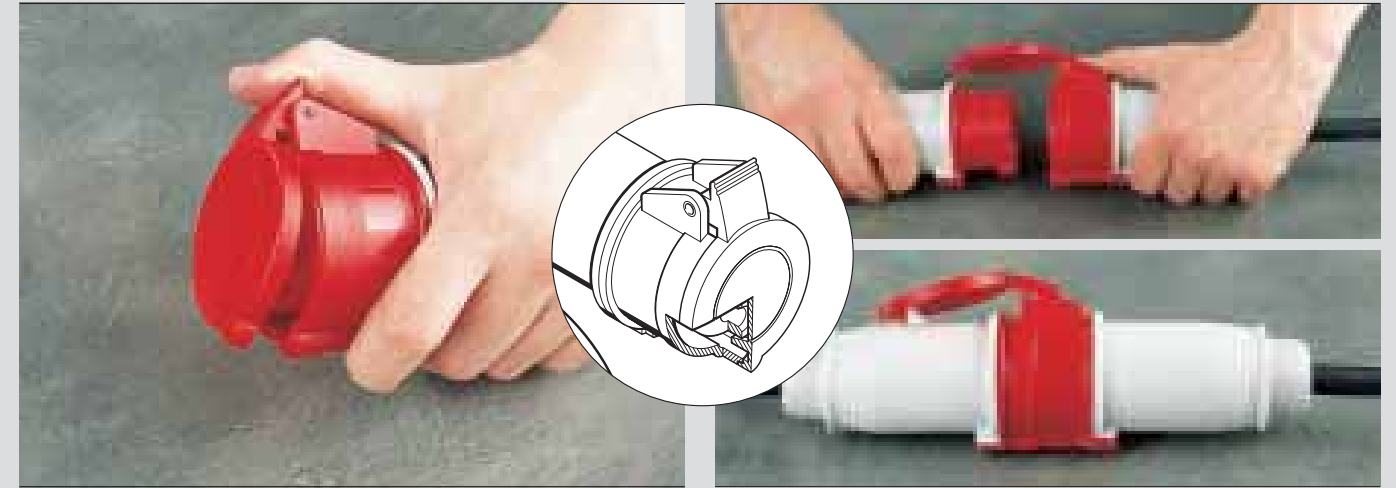
A wing on the lid assists one-handed opening. Splash-proof protection (IP44) is assured by the two inclined surfaces on the lid and on the insert. These surfaces also assist self-centring of the lid.
