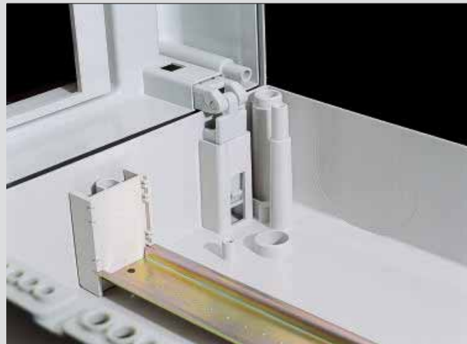
Hinges: should be snap-fitted into their guides, can be mounted on the left or the right side, in the series versions 12 to 64 DIN modules.
